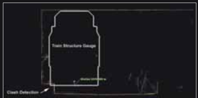
Application of train structure gauge in a point cloud cross section profile, Taipei Trupo Tunnel
